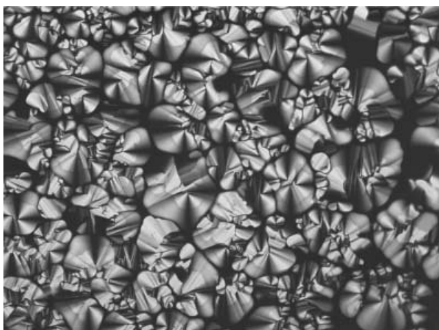
Figure 3. Mesophase texture of derivative 2i at 85°C, on cooling from the isotropic phase ( 0.5 \text{ K min}^{-1} , magnification 100\times ).
