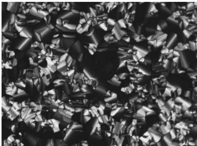
Figure 2. Mesophase texture of derivative 2e at 93°C, on cooling from the isotropic phase ( 5 \text{ K min}^{-1} , magnification 100\times ).
